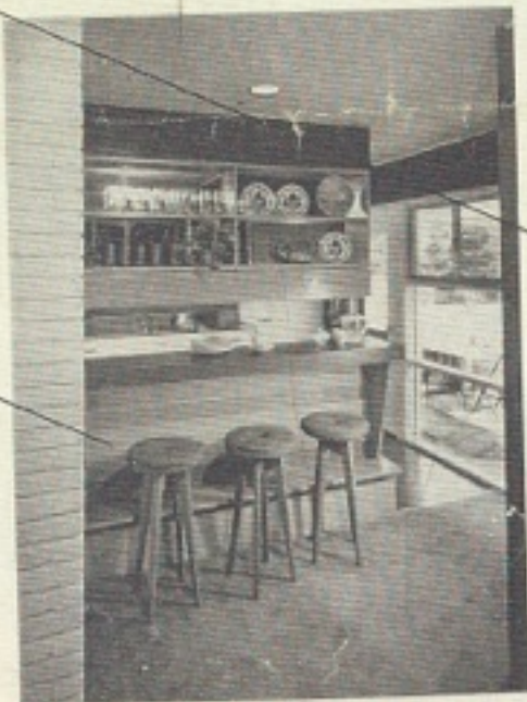
Bar-buffet is set in corner of living rooms, backing against kitchen. Counter opening can be closed by hinged panel, has mirror-backed shelves above. Kitchen area is lighted by 8-foot-wide window.
