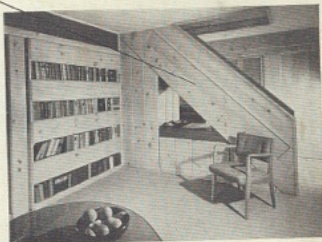
When closed, the 5½' x 7' hinged bookcase becomes living-room wall. Room behind has door to hall, may be used as bedroom. Bookcase, opened, converts it into a dining or study ell.
