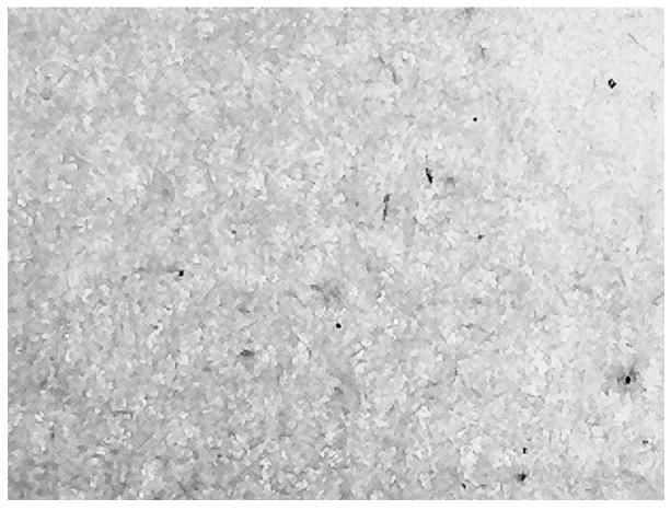
Paper made from wood pulp is characterized by short fibers and a very smooth, uniform surface.
