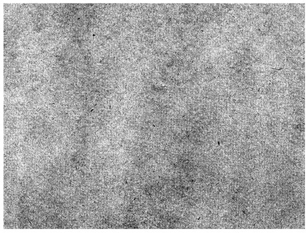
The mold used to produce wove paper is made of a very fine mesh which do not leave a distinctive impression in the paper. While the sheet is smoother than the laid paper, it still exhibits irregularity in the distribution of the cellulose fibers.
